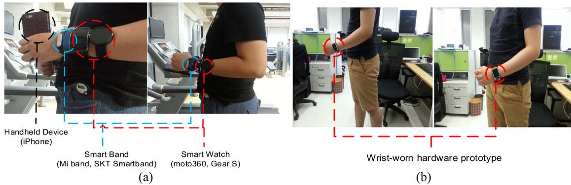
Fig. 13. Test conditions of commercial pedometers (a) and our hardware prototype (b).
