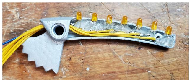
Close the wings with the covers and attach each with one 2,5 x 10 mm screw each. The 10mm screws still seemed a bit too long, but I could not get shorter ones, so I cut off the first ~2 mm of the screws prior to using them.
