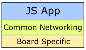
A JS App codes to an Espruino architected model of networking and the implementation of that common model invokes board specific implementation functions. For this to work, when we exchange one board specific implementation for another, the interfaces exposed by the board must be the same. What this means is that a board specific networking implementation must expose a "contract" that both sides agree upon.
