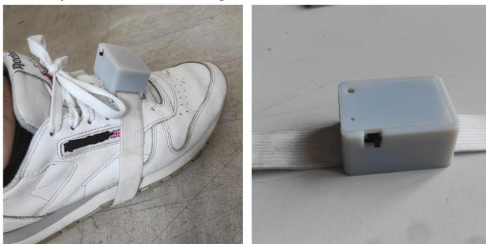
Figure 3.4 - IMU-based device inside the case
