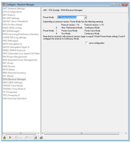
Figure 15: Receiver configuration for PSM
