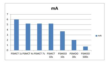
In a 10s update period it is advantageous from a current consumption point-of-view to use ON/OFF mode instead of cyclic tracking.
