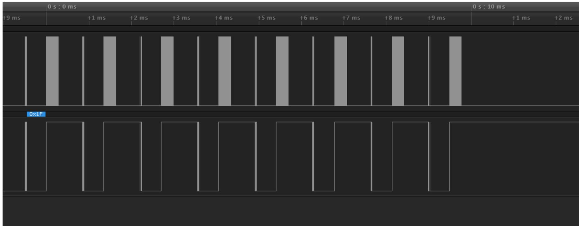
It appears that less than 50% of the SPI bandwidth is utilised. It is actually worse. If we zoom in once on an area of clock activity:
